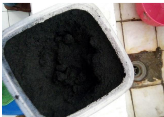
Figure 3 Bagasse activated carbon after activation and irradiation. (private collection)
